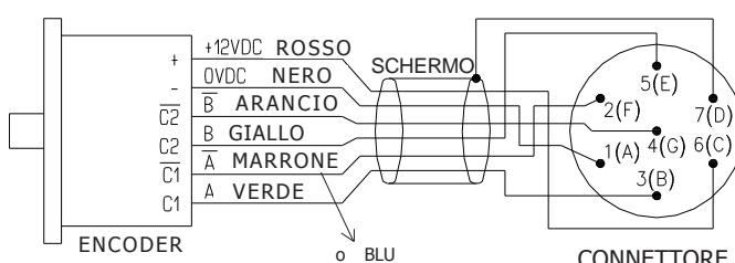
**encoder con impulso di zero**
